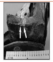
Close up view of the fracture location, at an area of two offset drilled holes (arrows).
